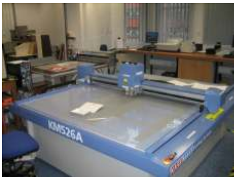
KM526A Cutting Table - KM Mount Cutter in background
